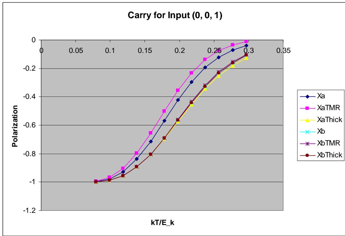
Fig. 19. Full Adder: Thermal performances on the carry output
