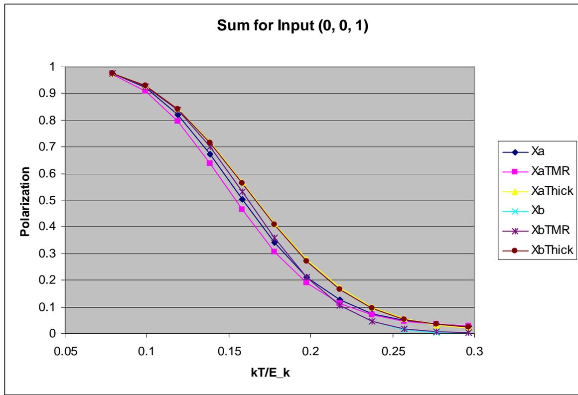
Fig. 20. Full Adder: Thermal performances on the Sum output
