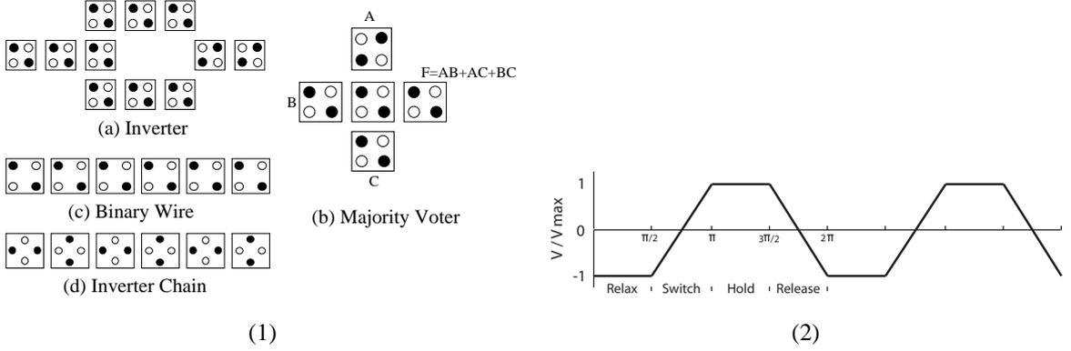
Fig. 2. (1) Basic QCA devices (2) Cmos-Clock-Signal
