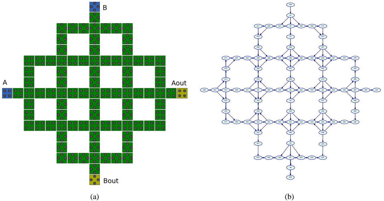
Fig. 8. 3 x 3 TMR crossing with rotated central cell (a) Layout (b) BN with 2-cell radius of influence.
