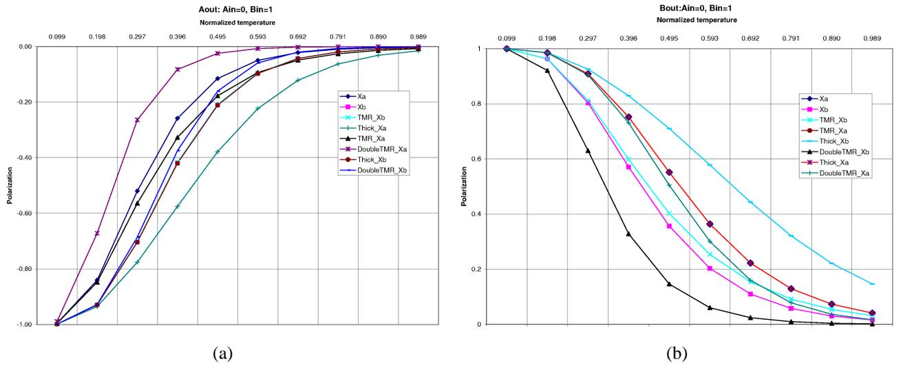
Fig. 14. Output polarization vs normalized temperature for  $A=0$   $B=1$  (a)  $A_{out}$  (b)  $B_{out}$
