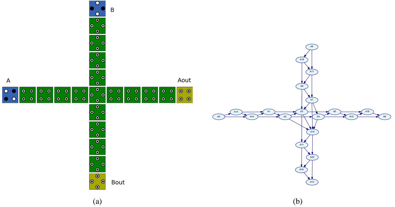
Fig. 5. Normal crossing with rotated central cell ( $Xa$ ) (a) Layout (b) BN with 2-cell radius of influence.
