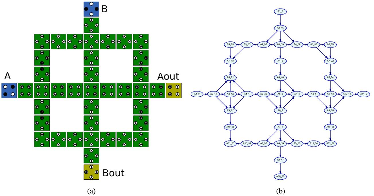
Fig. 7. 3x1 TMR crossing with non rotated central cell (TMRXb voting on the B line) (a) Layout (b) BN with 2-cell radius of influence.
