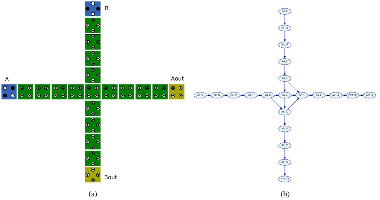
Fig. 6. Normal crossing with rotated central cell ( $Xb$ ) (a) Layout (b) BN with 2-cell radius of influence.
